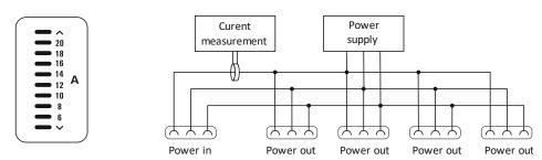
The bar graph LEDs show the total amps drawn by and through the XSH. The lighting down arrow led shows that the load is less than six amps if all other LEDs are turned off.
