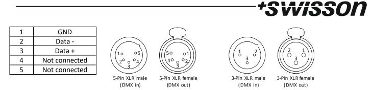
The DMX input is fully isolated and has a built-in termination. All outputs are isolated transmitters with a bias network for RDM operation. Each output port is individually optically isolated, meaning that it is totally isolated from the other output ports and from the input section.
