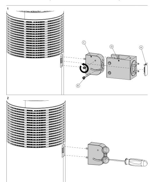
Remove the rubber from the desired side (A).
