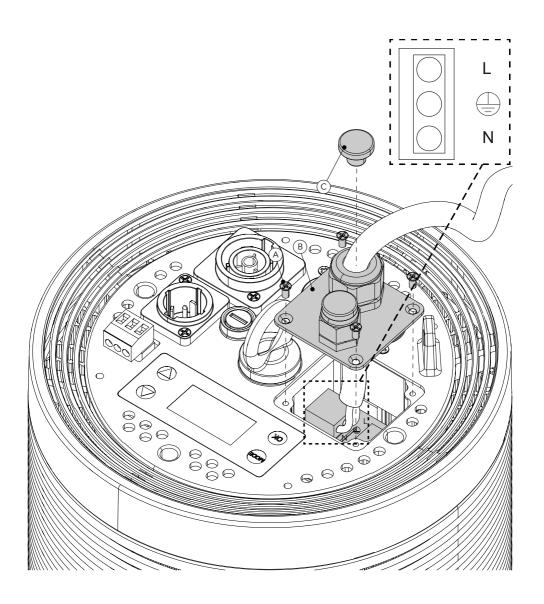
Loosen the four screws (A) and remove the plate with the cable glands (B). Loosen and remove the cap (C). Then insert the cable.
