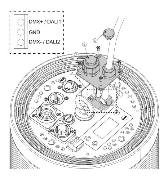
Loosen the four screws (A) and remove the plate with the cable glands (B). Loosen and remove the cap (C). Then insert the cable.
