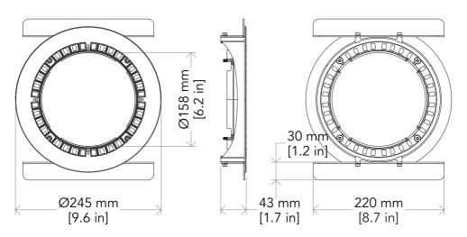
Measurements for cuts on the panels (1) and of Ceiling Recessed kit (2).
