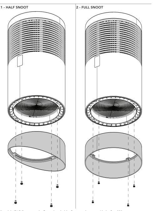
Attach half / full snoot to the fixture lens holder frame and secure with the four M4 screws.
