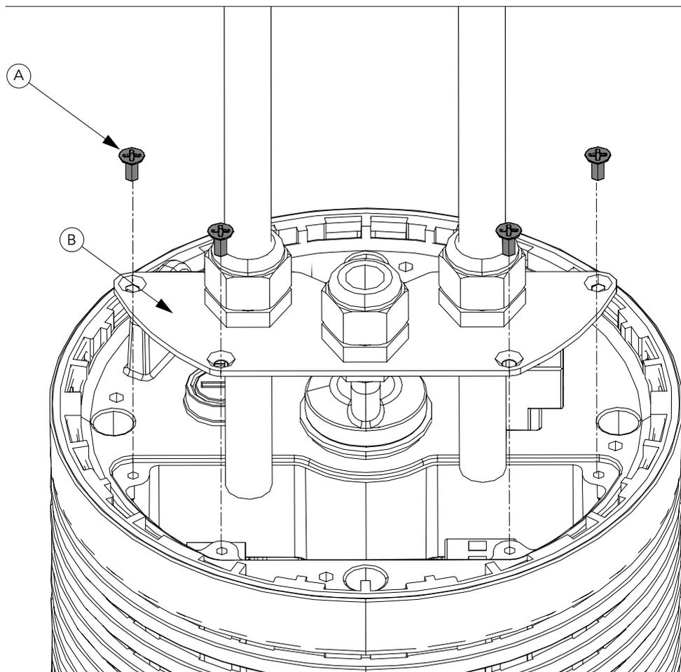
Loosen the four screws (A) and remove the plate with the cable glands (B). Then insert the cables.
