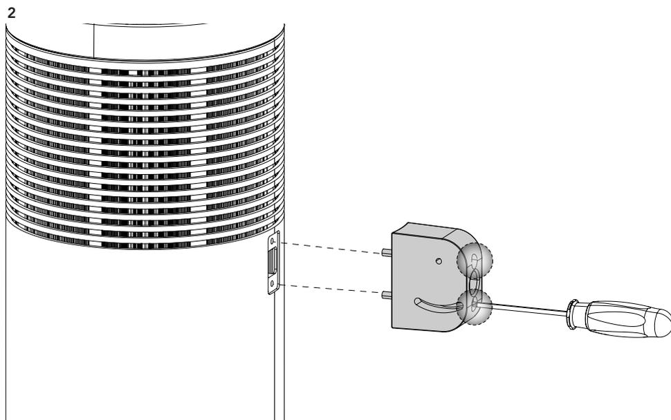
Remove the rubber from the desired side (A).
