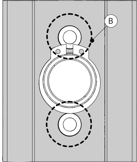
Rotate the disc (A) and align the two holes (B). Then insert the screws for wall fixing, and rotate it 90° again and insert the other two screws. Tighten the four screws in total.
