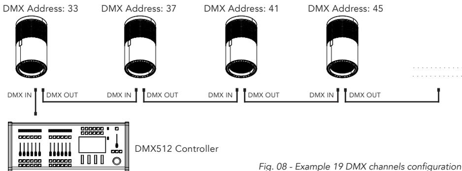
Fig. 08 - Example 19 DMX channels configuration
