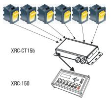
Each button can be configured to start, stop or pause, play back of a sequence on the XRC-150/200.
