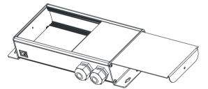
Now you can see the connecting ports (1 - 15) for the external trigger contacts and also two connectors of the internal power (VCC and GND):
