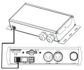
It doesn't matter on which port (port #1 or #2) the XRC-CT15b is connected to the XRC-150.
